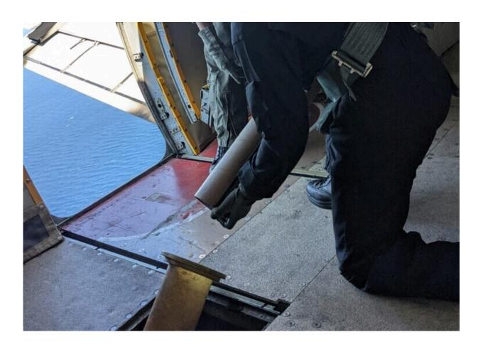
A "chute drop" of the microSWIFT technology, which aims the device directly down, during the Sept. 26 flight. Data from this instrument developed at the UW Applied Physics Laboratory will be combined with other observations to try and improve hurricane forecasts around the world. Credit: U.S. Navy/VXS-1 crew
