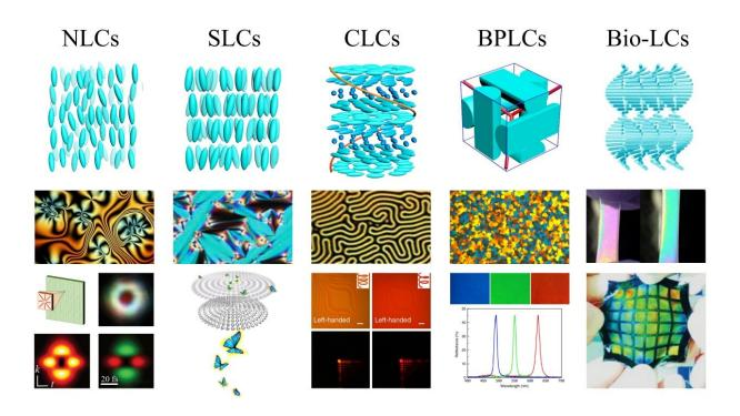
Schematic configurations, representative textures, and promising applications of nematic phase LCs, smectic phase LCs, cholesteric phase LCs, blue phase LCs, and bio-based LCs. Credit: Ling-Ling Ma, Chao-Yi Li, Jin-Tao Pan, Yue-E Ji, Chang Jiang, Ren Zheng, Ze-Yu Wang, Yu Wang, Bing-Xiang Li, Yan-Qing Lu
