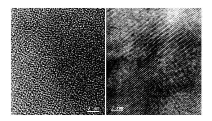
Images produced by transmission electron microscopy verified the transformation of the electrode material from a disordered arrangement of atoms (left) to an ordered, crystalline structure (right). Credit: Argonne National Laboratory
