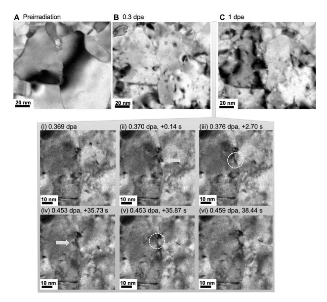
Evolution of the  $\Sigma 3$  GB during in situ TEM ion irradiation. (A) Preirradiation, (B) 0.3 dpa, and (C) 1 dpa. (i to vi) A series of still frames taken from in situ TEM. Movie S1 (0.369 to 0.459 dpa) illustrates the localized interaction between irradiation-induced defects (extrinsic to the GB) and the faceted  $\Sigma 3$  {112} GB. Credit: *Science Advances* (2022). DOI: 10.1126/sciadv.abn0900
