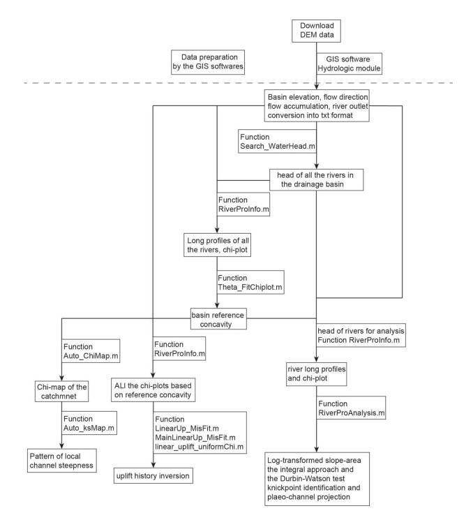
The flowchart tells the functions of the program and the input data and output results of each function. Credit: Science China Press
