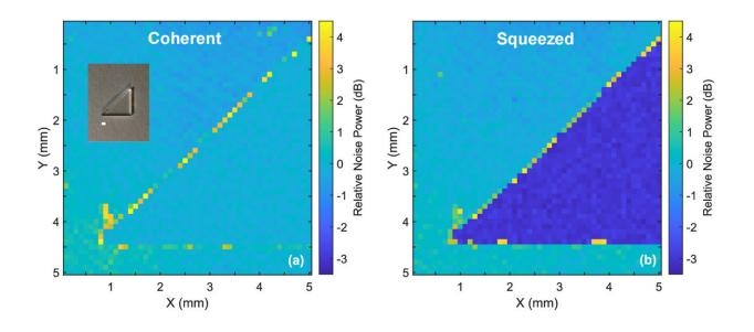
Quantum-enhanced microscopic imaging using water as the signal medium. The imaging object is a triangle-shaped piece of glass shown in the inset of (a), where the white scale bar is 1 mm in horizontal direction. More than 3 dB quantum-enhanced SNR, or image contrast, is clearly visible in (b). Credit: *Optica* (2022). DOI: 10.1364/OPTICA.467635
