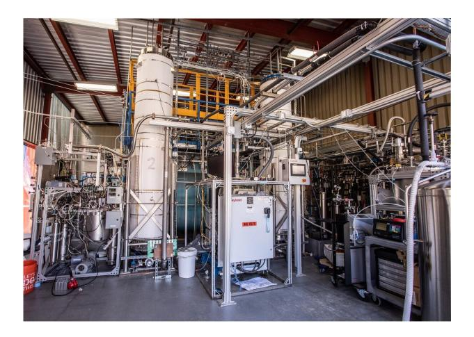
Xenon purification system at SLAC. The two central columns are each filled with almost half a ton of charcoal, which is used to produce ultra-clean xenon for the LUX-ZEPLIN (LZ) dark matter experiment. Credit: Jacqueline Ramseyer Orrell/SLAC National Accelerator Laboratory
