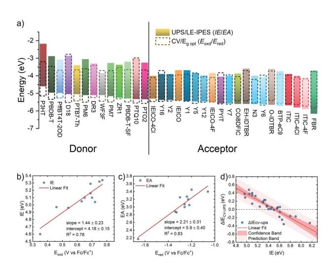
a) Energy levels of organic semiconductors measured using UPS, LE-IPES, and CV. b,c) Plots showing the correlation between  $E_{oxd}$  and IE (measured via UPS) (b), and  $E_{red}$  and EA (measured via LE-IPES) (c) of donor polymers. d) Scatter
