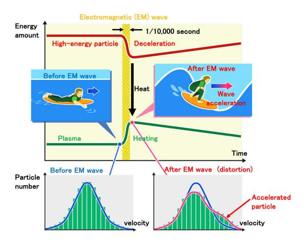
Heat is carried by electromagnetic waves, which simultaneously slow down the high-speed particle beam (red line) and heat up the plasma particles (green line). Distortion of the velocity distribution is observed due to the acceleration of the particles as a result of the electromagnetic waves. Credit: National Institute for Fusion Science
