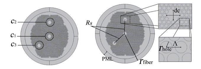
The three-core optical fiber sensor designed by the researchers for measuring spine curvature. The position of the three fiber cores creates an asymmetric geometry in the proposed sensor, allowing it to measure both the direction and magnitude of the spine curvature. Credit: *Optical Engineering* (2022). DOI: 10.1117/1.OE.61.9.097102
