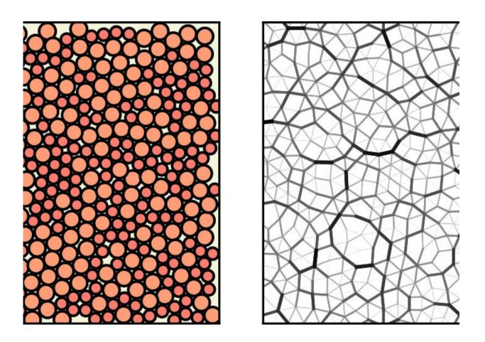
Configuration of a typical granular solid (left hand side). The force network or force chain in such a material is shown on the right hand side. Credit: Rituparno Mandal
