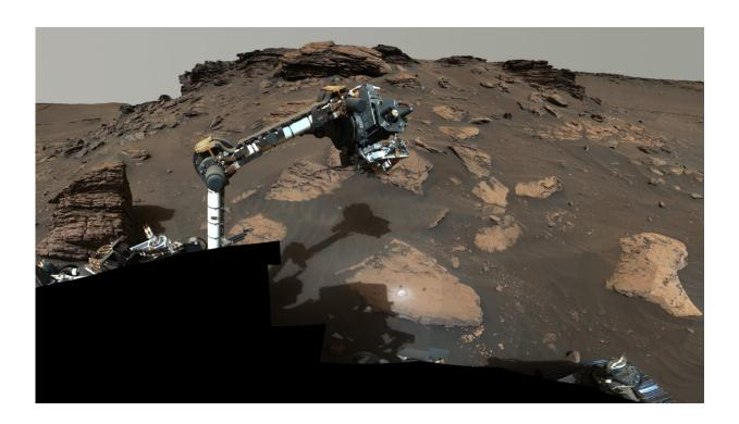
NASA's Perseverance rover puts its robotic arm to work around a rocky outcrop called "Skinner Ridge" in Mars' Jezero Crater. Composed of multiple images, this mosaic shows layered sedimentary rocks in the face of a cliff in the delta, as well as one of the locations where the rover abraded a circular patch to analyze a rock's composition. Credit: NASA/JPL-Caltech/ASU/MSSS
