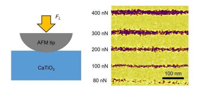
Left: Data storage using probe force. Right: Data storage area drawn with a width of 10 nm or less. Credit: POSTECH
