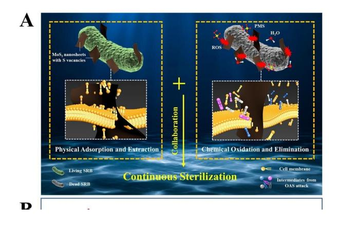
Fig. 1 (A) Schematic illustration of the continuous anaerobic bactericidal mechanism via physical extraction and chemical oxidation; (B) PMS and H2O adsorption on (001) surface of SVs-MoS2. Credit: IOCAS
