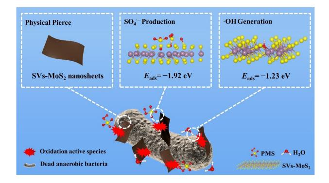
Fig. 2 The scheme of the collaboration of physical pierce and chemical injury of MoS2 nanosheets. Credit: IOCAS
