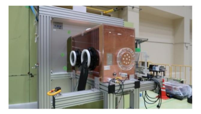
The custom-made experiment setup developed to avoid the samples from being contaminated by the Earth's atmosphere. The interior is filled with helium gas, and the chamber is lined with pure copper to minimize background noise. Credit: Muon analysis team
