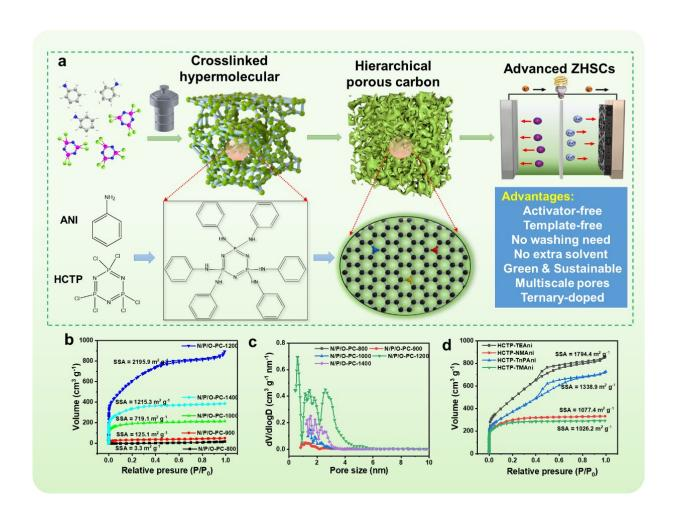
(a) Schematic illustration of the fabrication processes of the carbons and the advantages of this method; (b) the nitrogen adsorption/desorption isotherms and (c) the corresponding pore size distribution curves; (d) nitrogen adsorption/desorption isotherms of the carbons obtained from other molecular precursors. Credit: Science China Press
