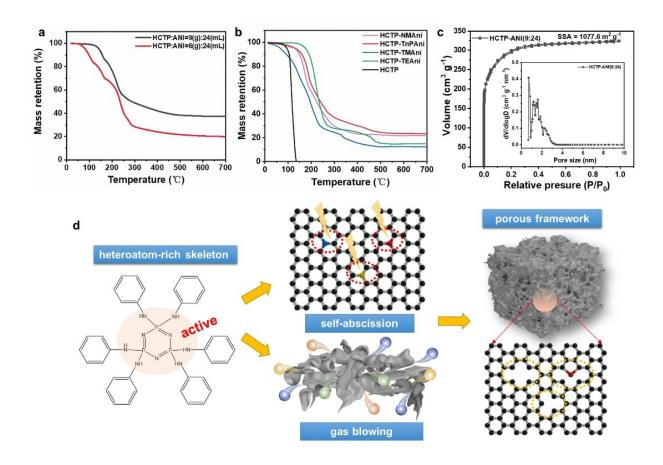
(a, b) TGA curves of different molecular precursors; (c) nitrogen adsorption/desorption curves and the pore size distribution curve of the carbons obtained under high addition ratio of the branched units; (d) schematic illustration of the pore formation mechanism. Credit: Science China Press
