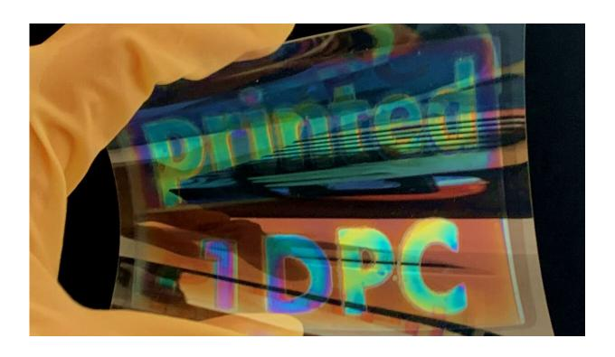
Colored mirror layer printed onto a foil. Inkjet printing allows for structurization, such that large-area logos can be printed as well. Credit: Qihao Jin, KIT
