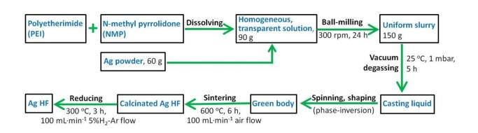
Diagram of the detailed fabrication procedures of Ag HF. Credit: *Angewandte Chemie International Edition* (2022). DOI: 10.1002/anie.202210432
