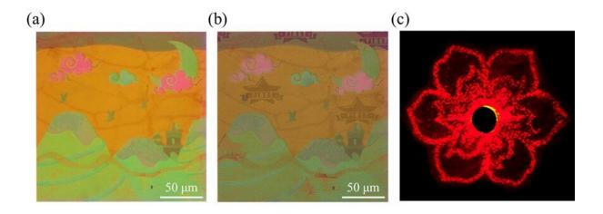
Researchers have developed a metasurface device that can display three types of images depending on the illumination light. Shown are a color nanoprinted image (a), the same image with a polarization-dependent watermark (b), and a holographic flower (c). Credit: Qi Dai, Wuhan University
