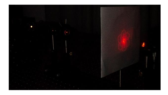
For the experiment, the holographic images were visualized using an optical path consisting of a continuum laser, iris, lens, the sample and an optical screen. Credit: Qi Dai, Wuhan University
