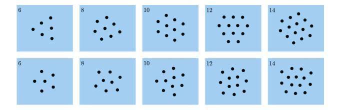
Different assemblies of N particles on the surface of the liquid. For each number N of particles, two different assemblies are shown opposite each other, demonstrating the metastability of the assembly. Credit: Université de Liège /N.Vandewalle
