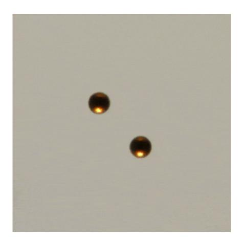
Animation of the growth of a floating crystal from N=3 to N=19 particles. Particles are added one by one to the surface of the liquid under magnetic field. The attractive capillary forces are counterbalanced by the repulsive magnetic forces. The assembly shows a symmetry typical of atomic crystals. Credit: Université de Liège / N.Vandewalle
