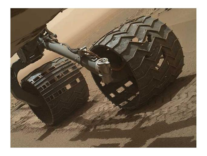
The wheels of the Curiosity rover have taken damage over the years, leaving behind small bits of aluminum. Credit: NASA/JPL-Caltech
