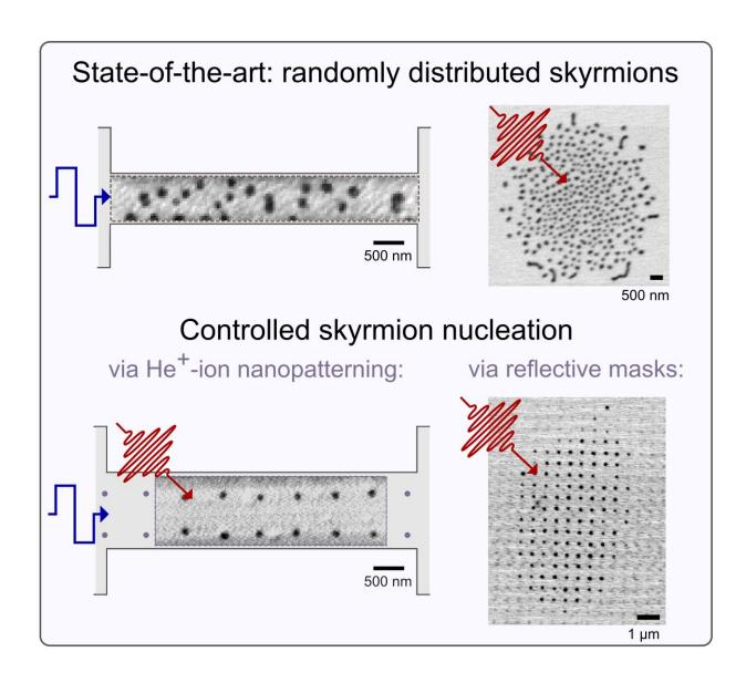
Figure 1: From randomly distributed skyrmions to nanometer position control in magnetic thin films: Two approaches either employing helium-ion irradiation or
