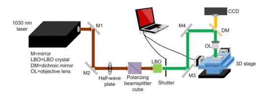
Figure 1. Schematic of laser fabrication system for microfluidic SERS chips. Credit: Compuscript Ltd
