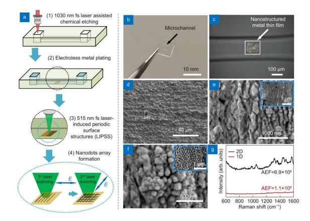
Figure 2. (a) Schematic of the fabrication (b) Photograph of microfluidic SERS chip (c) Optical microscope image showing the SERS substrate. SEM images of (d) original metal film, (e) ripples generated by 1st laser scanning and (f) nanodots generated by 2nd laser scanning (Insert: low magnification of SEM image). (g) Raman spectra of 10-9 M Rhodamine 6G (R6G) on 2-D (black) and 1-D (red) nanostructured SERS substrates. Credit: Compuscript Ltd
