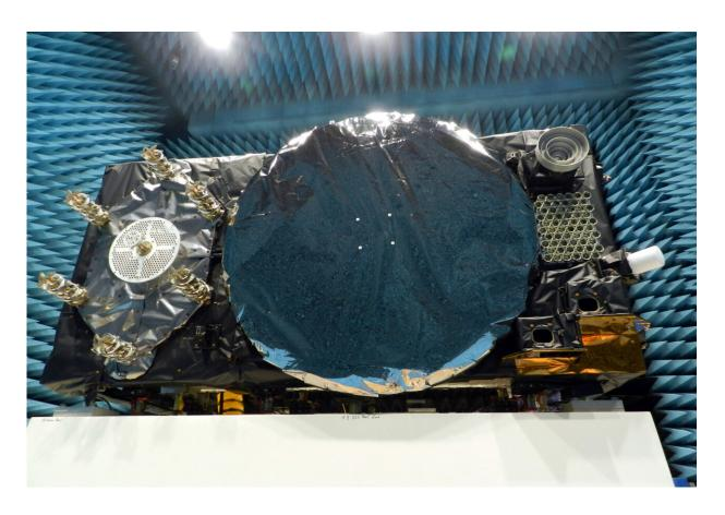
Seen here sheathed in multi-layer insulation, the 2.5m by 1.2 m by 1.1 m satellite's main 1.4-m diameter antenna transmits L-band navigation signals down to Earth. To its left is the hexagonal search and rescue antenna that picks up distress signals and relays them to local emergency services, contributing to the saving of more than 2000 lives annually. Credit: European Space Agency
