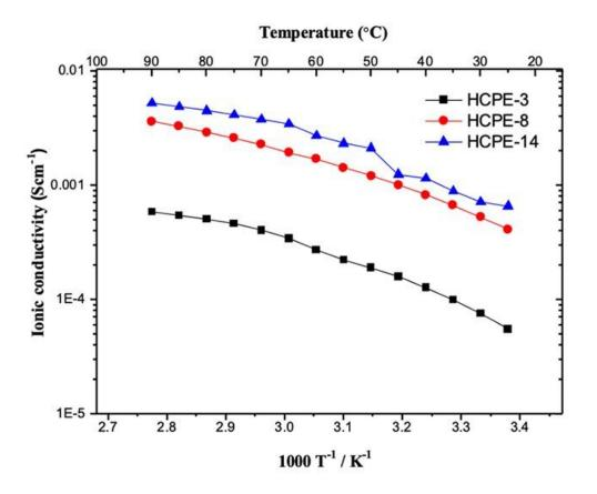
Temperature dependences of different pore size honeycomb film composite electrolytes on ionic conductivities. Credit: Grewal and Yabu
