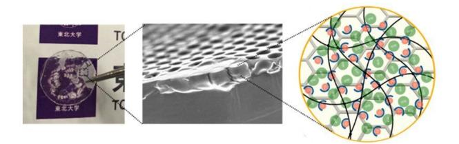
A photograph (left), scanning electron microscope image (center), and schematic illustration of composite electrolyte structure (right), respectively. Credit: Grewal and Yabu.
