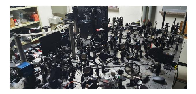
Figure 1. Super-depth 3D holographic microscope A super-depth 3D holographic microscope developed by researchers at the IBS Center for Molecular Spectroscopy and Dynamics. It is possible to observe the neural network of living organisms by increasing the target optical signal ratio and increasing the image acquisition speed and depth. Credit: Institute for Basic Science
