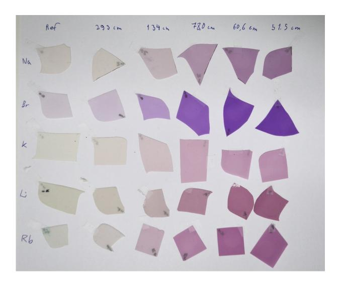
Hackmanite plates that have changed color upon radiation in the laboratory of the Finnish Radiation and Nuclear Safety Authority. The plates show the
