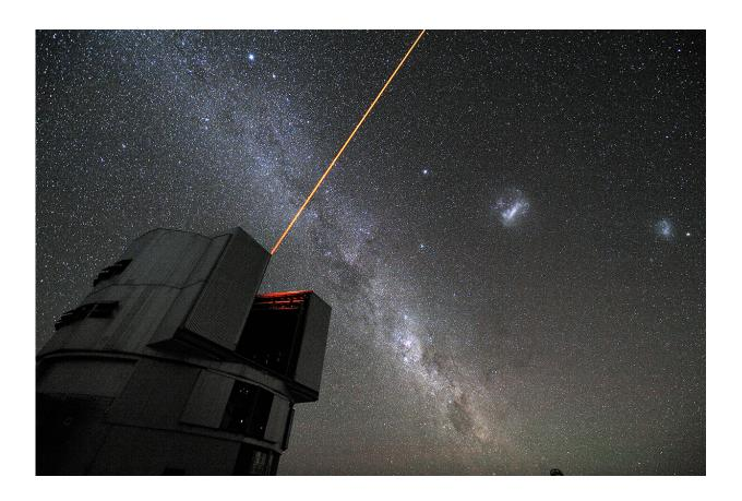
The VLT's Laser Guide Star: A laser beam launched from VLT's 8.2-meter Yepun telescope crosses the majestic southern sky and creates an artificial star at 90 km altitude in the high Earth's mesosphere. The Laser Guide Star (LGS) is part of the VLT's Adaptive Optics system and it is used as reference to correct images from the blurring effect of the atmosphere. Credit: ESO / G. Hüdepohl (atacamaphoto.com)
