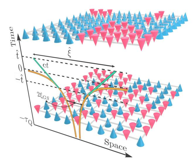
Schematic depiction of the dynamics across a phase transition in a twodimensional spin-1/2 model. In the initial paramagnetic state (bottom), spins align with the direction of the transverse magnetic field. A measurement of the spin configuration in that state along the ordering direction would then typically
