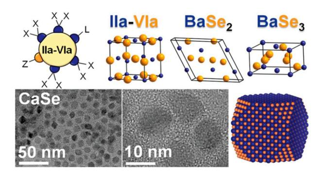
Unit cells and electron micrographs of alkaline-earth chalcogenide (AeCh) nanocrystals. Credit: U.S. Department of Energy Ames National Laboratory
