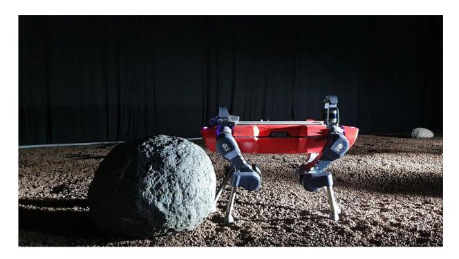
LEAP (Legged Exploration of the Aristarchus Plateau) is a mission concept study funded by ESA to explore some of the most challenging lunar terrains. Credit: ETH Zürich/RSL Robotics Labs
