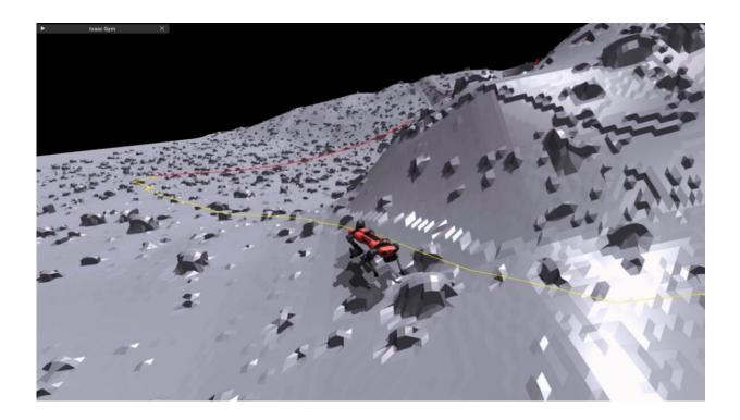
The LEAP rover is trained using a Reinforcement Learning approach in a virtual environment to simulate the lunar terrain, gravity and dust properties. Credit: ETH Zürich/RSL Robotics Labs
