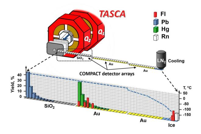
Schematic view of experiment setup. Credit: A. Yakushev, GSI/FAIR
