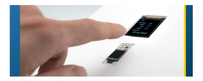
Secure and noninvasive fingerprint biosensor can detect molecules circulating in the body. Credit: UCLA/Interconnected & Integrated Bioelectronics Lab
