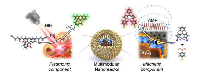
Schematic diagram of the magnetic-plasmonic catalytic multimodular nanoreactor. Credit: POSTECH
