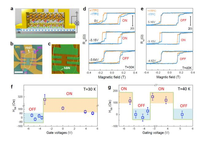
(a) Schematic of the solid proton field effect transistor. (b, c) Optical and atomic force microscope images of heterostructure device. (d, e) Gate-dependent exchange bias effects at T = 30 and 40 K, respectively. (f, g) Amplitudes of the exchange bias effects under various gating voltages at T = 30 and 40 K, respectively. Credit: Zheng Guolin
