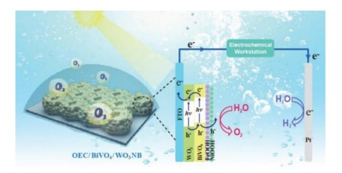
As one of the most promising photoanode candidates for photoelectronchemical water splitting, the photocurrent density and IPCE of BiVO4 have been improved to 5 times higher by constructing OEC/BiVO4 and highly matched BiVO4/WO3 nanobowl "multiple junctions." Credit: *Chinese Journal of Catalysis* (2022). DOI: 10.1016/S1872-2067(21)63927-X
