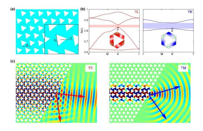
Dual-polarization valley photonic crystals. (a) Structure of the valley photonic crystal, (b) Bulk band structure and eigen fields of representative bulk modes at the K point. (c) Polarization dependent refraction of edge modes. Credit: Science China Press
