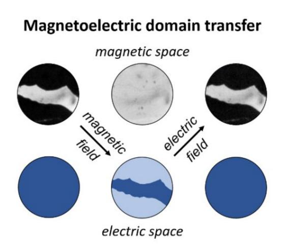
Magnetoelectric domain transfer. The application of a magnetic field translates a magnetic domain pattern into a ferroelectric pattern, while simultaneously erasing it in the magnetic state. An electric field reverses the process. The
