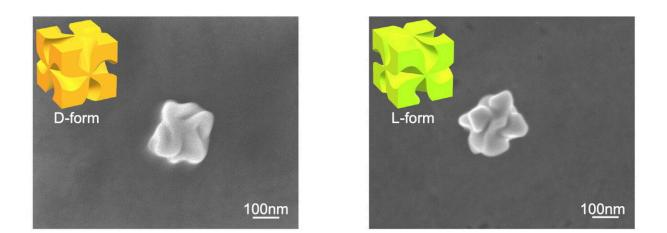
Scanning electron microscopy images show D- and L- form gold chiral nanoparticles. The insets visualize the three-dimensional models of the nanoparticles. Credit: NINS/IMS
