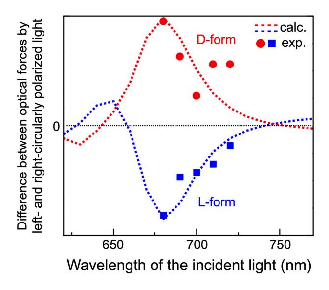
The plots are the experimental data and broken line are the theoretical calculation. Red and blue in the plots and line represents the D- and L-form nanoparticles, respectively. The optical gradient force was different for D-form and L-form particles. Credit: NINS/IMS
