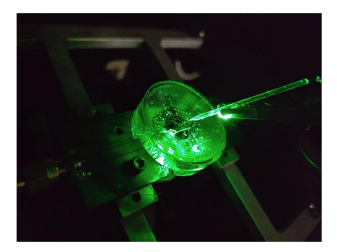
A prototype of a diamond voltage imaging microscope constructed by physicists at the University of Melbourne. A tiny electrode is suspended above the diamond chip to test the performance of the device. A green laser shone from below provides fluorescence excitation to the chip. Credit: Author provided, University of Melbourne
