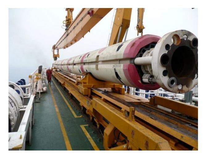
A drilling riser aboard the scientific drilling vessel Chikyu. Dozens of risers were linked together to reach deeper into an earthquake fault than ever before. Led by researchers at the University of Texas Institute for Geophysics and University of Washington, the scientific mission revealed that tectonic stress in Japan's Nankai subduction zone was lower than expected. Credit: Demian Saffer/University of Texas Institute for Geophysics
