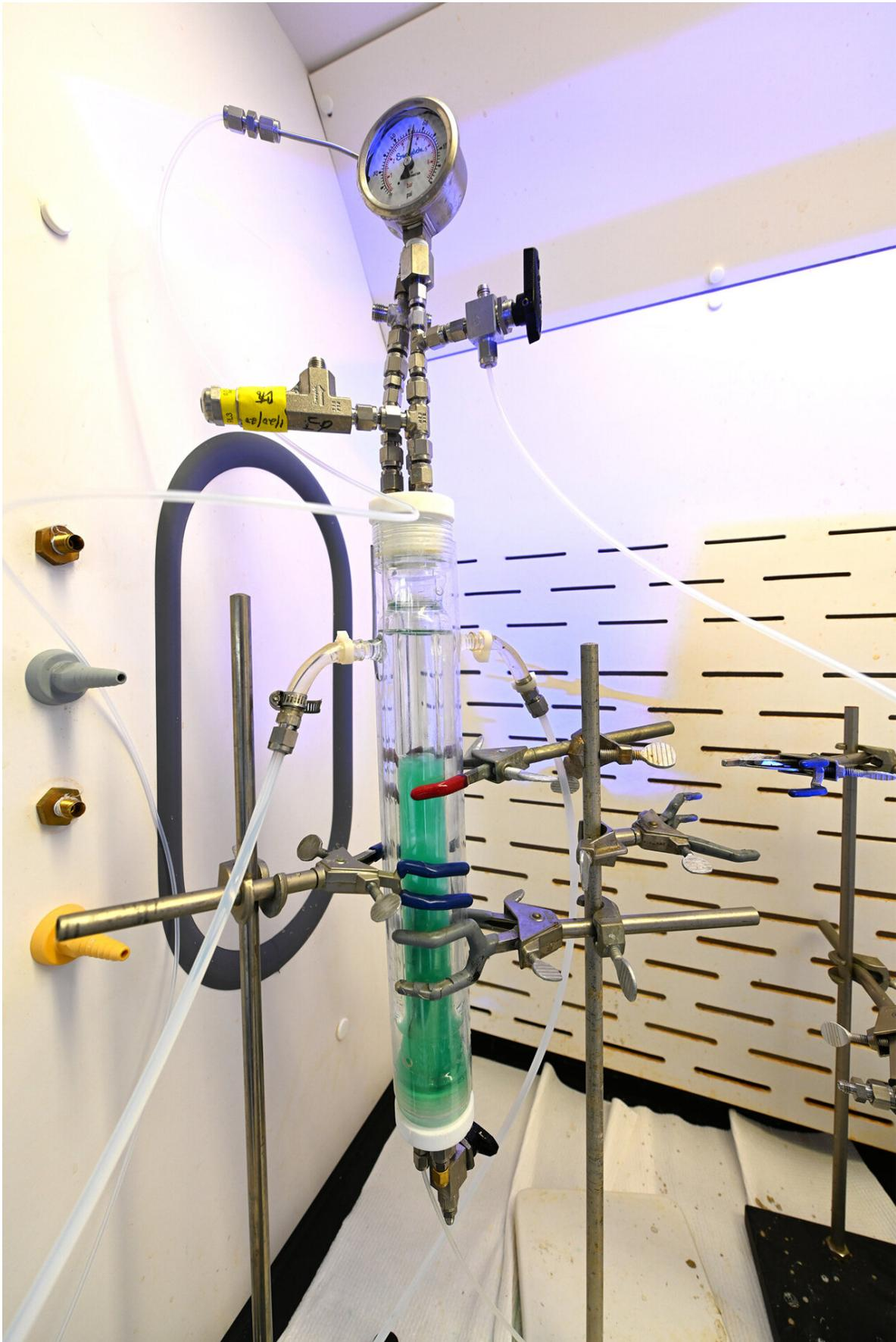
The contraption used to filter out different chemical components in these spent magnets. Credit: Idaho National Laboratory
