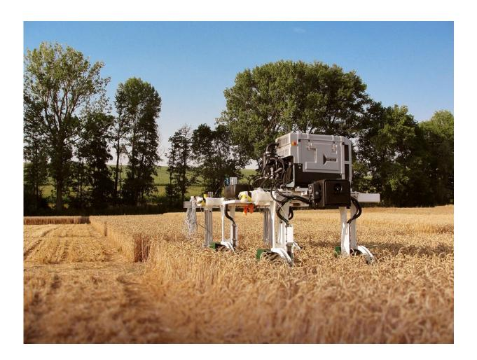
The field robot DeBiFix examines whole wheat fields to show how the kernels are developing inside the ears. This can be used as a basis to determine which varieties are particularly suitable for breeding. Credit: Fraunhofer IIS
