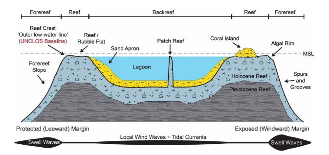
Cross-section of coral reef geomorphic zones, showing wave energy gradients,
