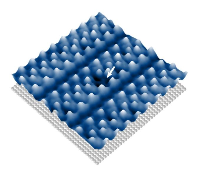
How the catalytically active molecules arranged themselves into almost perfect single-layer structures on a polished silver surface. Credit: Ole Bunjes
