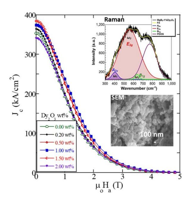
The low and high field critical current density of bulk MgB<sub>2</sub> superconductors can
