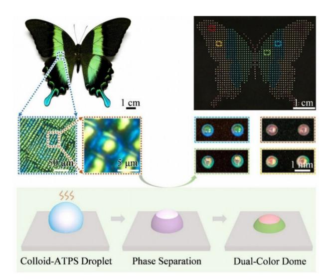
Taking advantage of the evaporation-induced phase separation of ATPS, biomimetic dual-color domes are fabricated by drying an ATPS droplet that contains mono-sized nanoparticles. Credit: The University of Hong Kong
