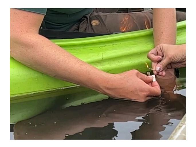
Turning the valve on the bubble trap releases methane gas, which is flammable. Holding a match near the valve ignites the gas in a burst of flame. Credit: NASA / Sofie Bates
