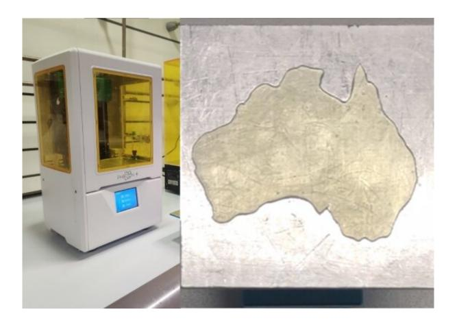
Researchers at UNSW Sydney used a standard 3D printer to produce an intricate map of Australia made of solid polymer electrolyte which was then tested as an energy storage device. Credit: Dr Nathaniel Corrigan
