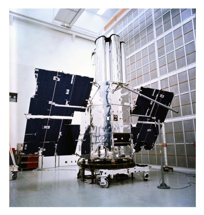
Orbiting Astronomical Observatory C – named Copernicus in orbit – stands in the Hangar AE clean room at Cape Canaveral Air Force Station, Florida, following the mounting of its stationary solar panels. Copernicus was the only member of the series sporting the large cylindrical structures at the top of the spacecraft, which kept stray light from reaching the instruments. Credit: NASA
